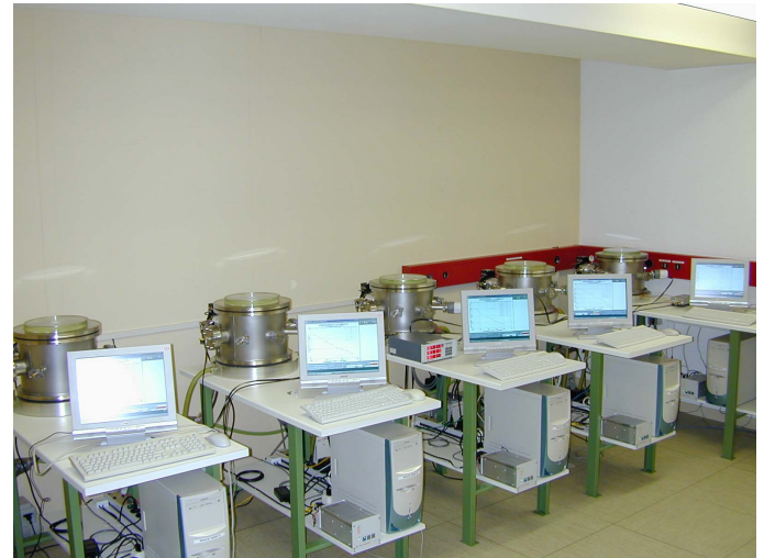
Figure 3. The five vacuum chambers used for lifetime test.
